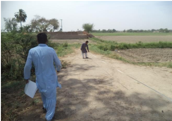
Plate 44: Measurement of off-set for area cropped is being measured along the road alignment.
