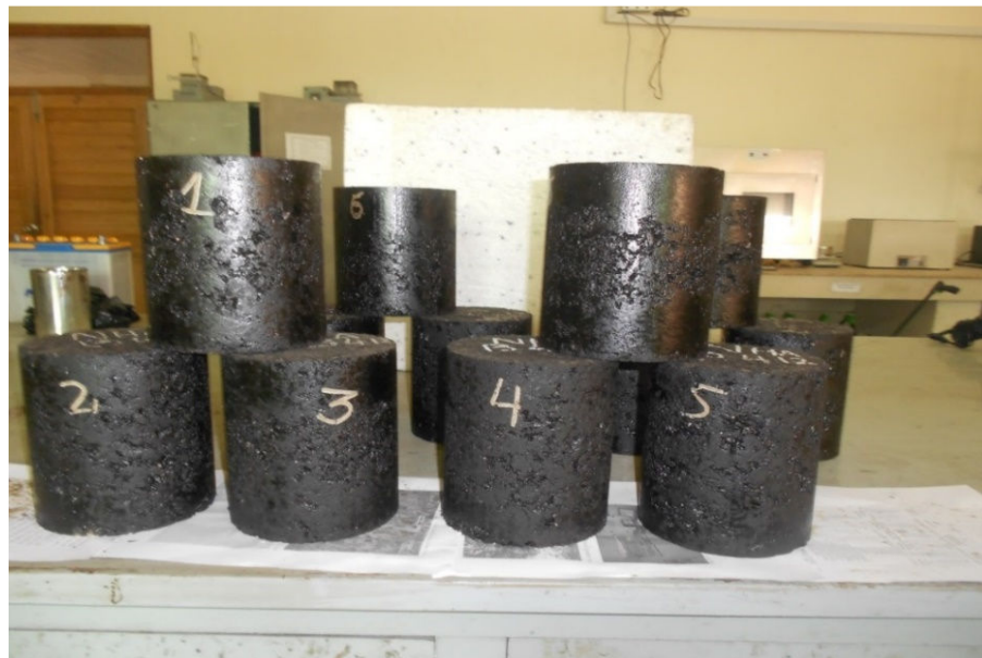
Figure 5.1: Specimen Prepared Using Gyrotory Compactor
