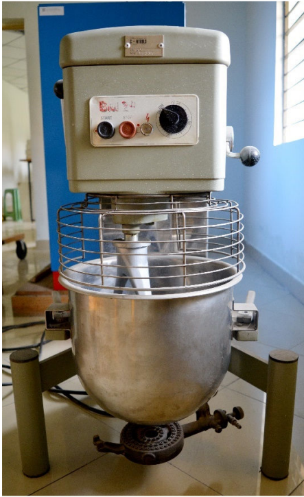
Figure 3.20: Electric Mixer to blend Aggregate and Bitumen
