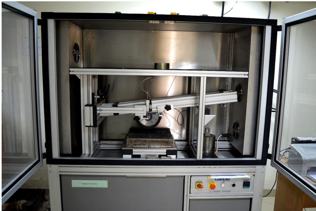
Figure 4.6: Cooper Wheel Tracker
