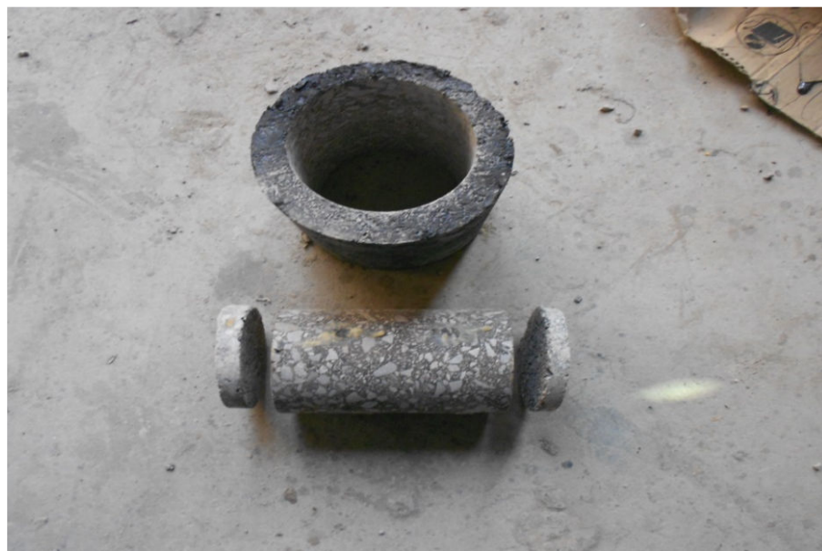
Figure 5.2: Cored and Trimmed Specimen with Waster Rings
