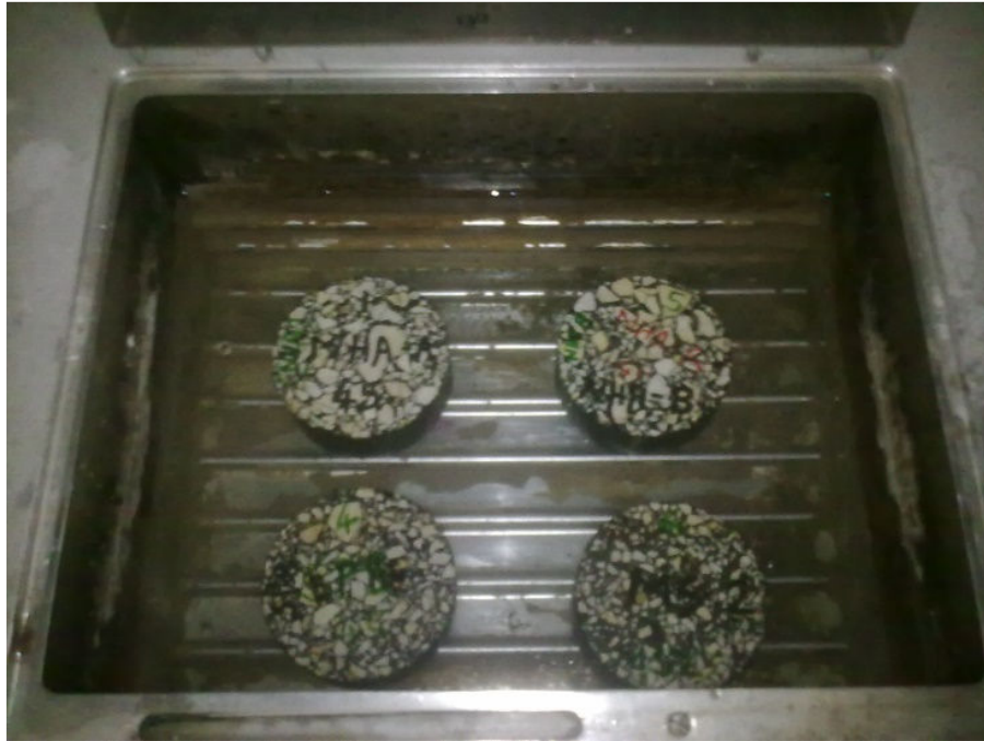
Figure 9.2: Moisture Conditioning of Samples in Water Bath
