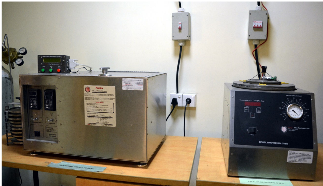
Figure 3.5: Pressure Ageing Vessel (PAV)
