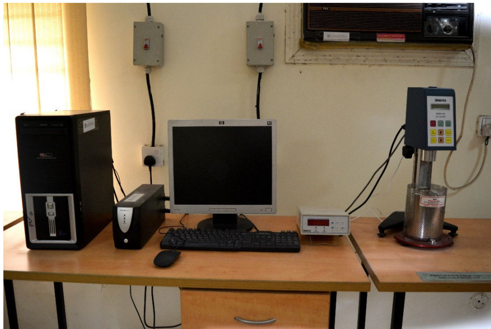
Figure 3.6: Rotational Viscometer (RV)
