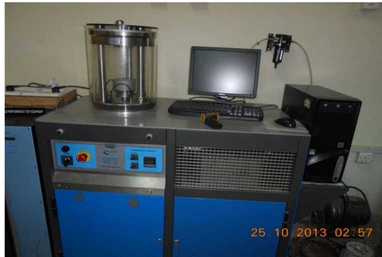
Figure 5.5: Simple Performance Tester (SPT)
