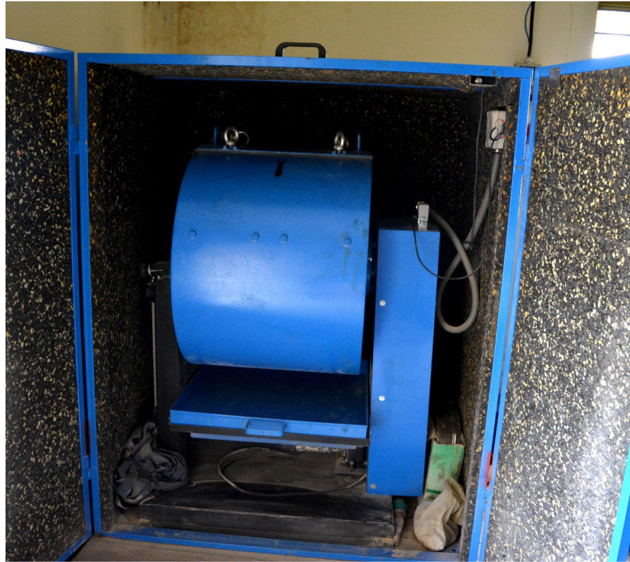
Figure 3.1: Los Angeles Abrasion Test Equipment
