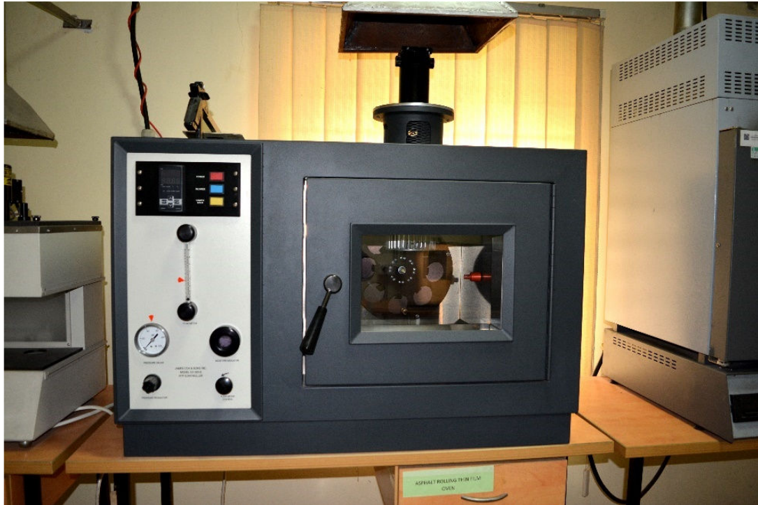
Figure 3.4: Rolling Thin Film Oven (RTFO)
