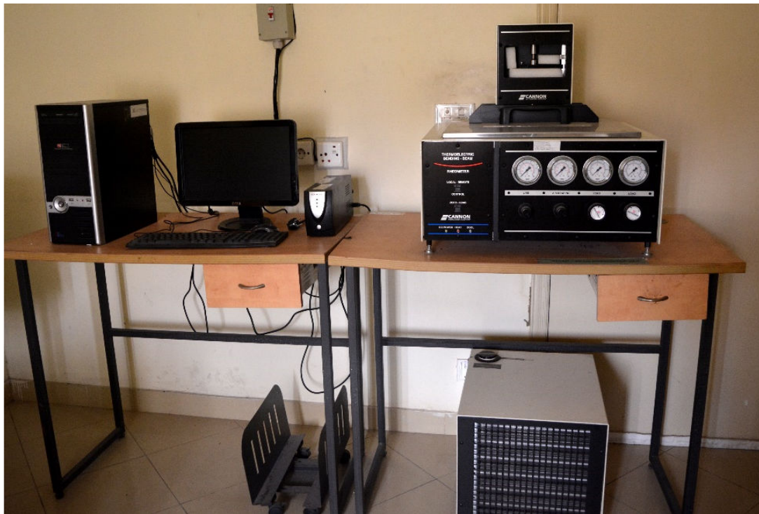
Figure 3.8: Bending Beam Rheometer (BBR)
