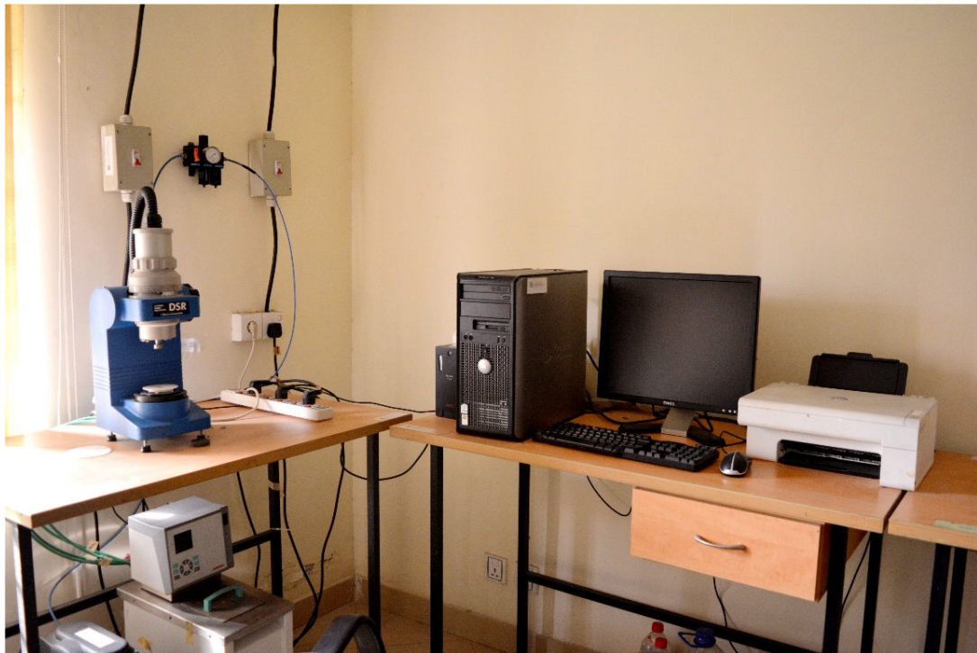
Figure 3.15: Dynamic Shear Rheometer (DSR)
