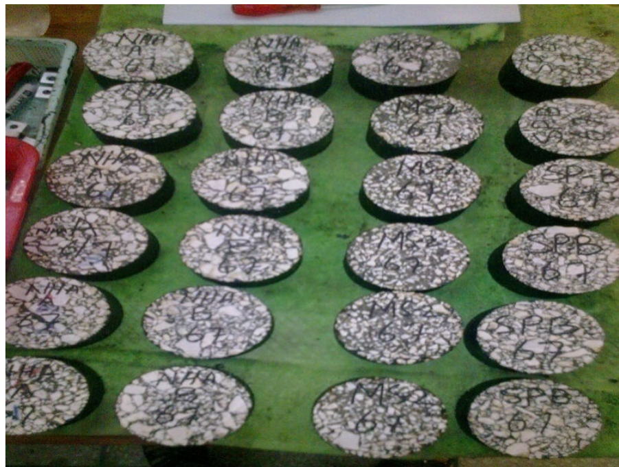
Figure 9.1: Samples Prepared for Moisture Conditioning
