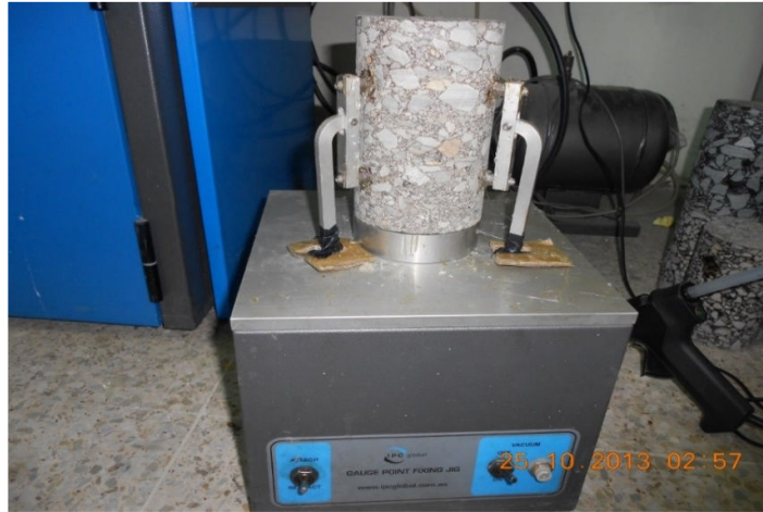
Figure 5.3: Gauge Point Fixing Jig
