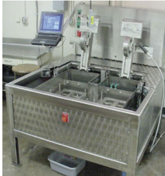
Figure 2.11: Hamburg Wheel Tracker
