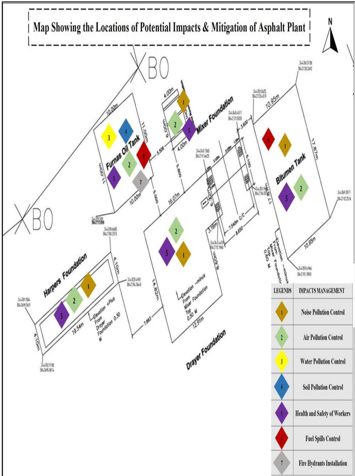
**Figure 4-3(b): Map Showing The Location Of Mitigation Measure At Asphalt Plant**
